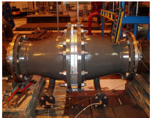
Figure 2: The Prototype used to test for flow and pressure drop performance
