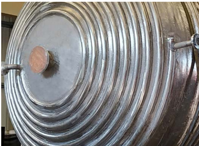
Figure 1 Limpet Coils are welded to the bottom and sides of the pressure vessel
