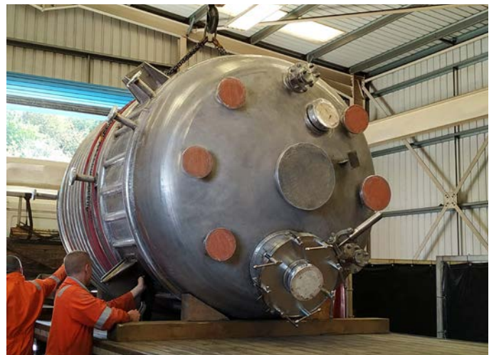
Figure 2 Limpet Coil Vessel being loaded for delivery
